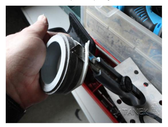
We pass all the disc to finish the edge of the ring of the valve.
