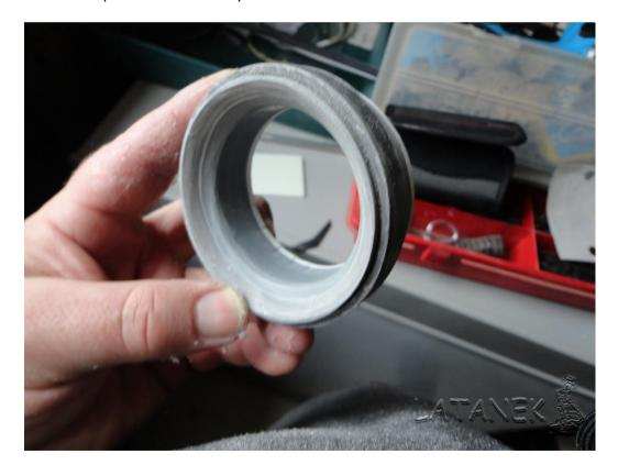
On the piece remaining sheet of PVC foam. Asked the valve and drawing pencil brand outside and inside of the valve, and then positioned trademarks for drilling the mounting holes.
