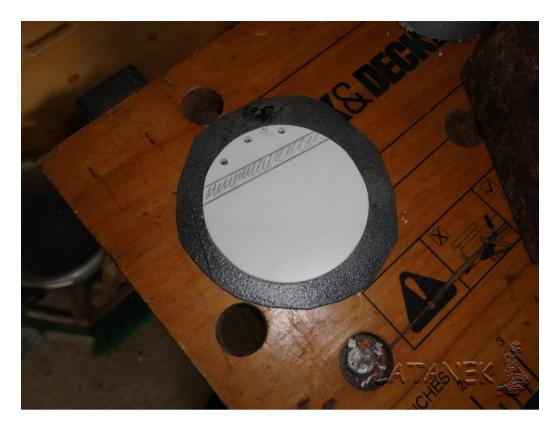
Once stuck, carefully cutting the edge of the valve and then set the cutter so that the saw blade ensure that 2.5 to 2.7 mm for cutting the hinge this CI is very IMPORTANT otherwise you'll have to redo a valve plate.
