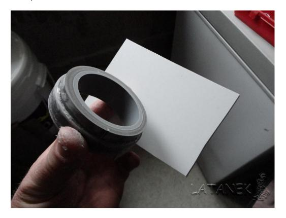
We'll paste this sheet of pvc on the valve and it puts a top weight to ensure a good contact and proper sealing.
