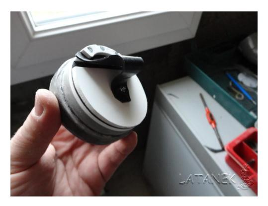
There is an adjustment to make, trim the edges of the valve for a full opening in the tube. The seal provided by the recovery and the flexibility of the rubber
