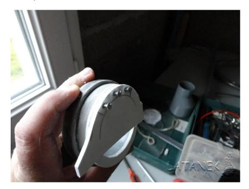
Size is another piece in the expanded PVC plate and drilling the holes with a 3mm drill.
