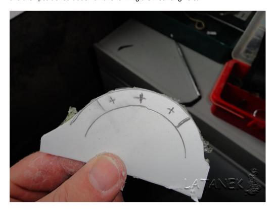
Positioned on the valve plate and drilling 3 holes with 2.5 mm drill without moving the whole then drill the holes of the plate only with 3 mm drill bit
